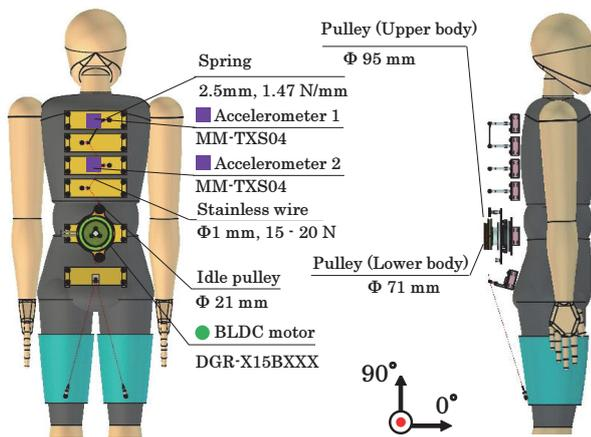
Fig. 1. Configuration of power-assisted lumbar suit.
