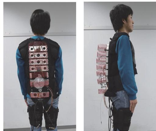
Fig. 2. Appearance of developed assist suit.
