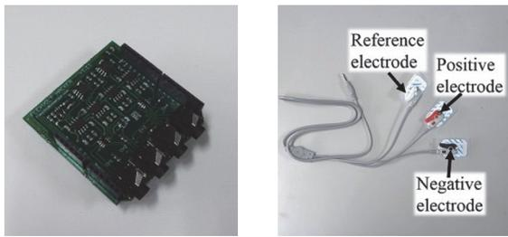
(a) Amplifier board (b) Myoelectric pads
