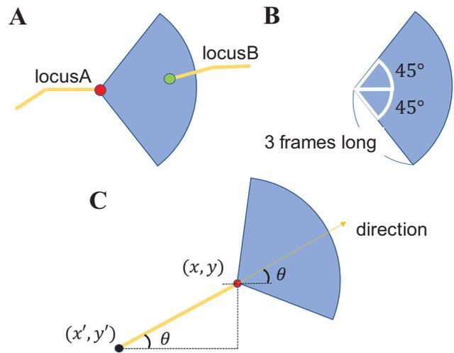
**Fig. 3.** (A) Fan shapes showing the predicted region of movement in a few frames. After a nearest-neighbor search, locus A and locus B are generated. These are shown by yellow lines. Within the fan-shaped region predicted from the endpoint of locus A, there is a locus B that starts several frames later. In this case, locus A and locus B are considered to be the trajectories of the same individual. (B) The fan shape. (C) Fan-shaped installation direction standard.
