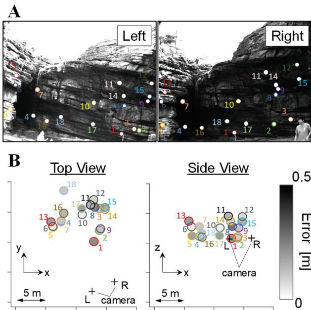
**Fig. 2.** (A) Photographs taken by the left and right cameras, including calibration points. (B) Color maps of measurement errors of 3D coordinates in manual analysis of observation space from top (left) and side (right) views.
