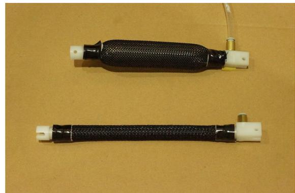
Fig. 1. Overview of MPA at normal state (bottom) and contraction state (top).
