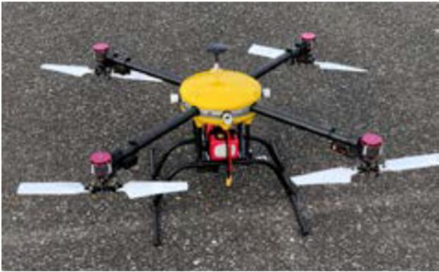
Fig. 1. Pitch-controlled quadrotor drone [11].
