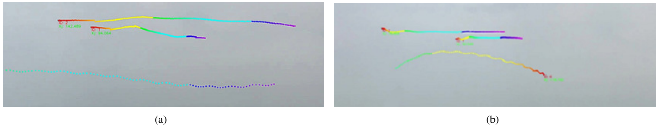
Fig. 4. Snapshot from the video clip of the two tracked drones flying above one tracked bird below with their trajectories.
