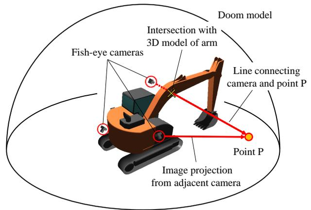
Fig. 5. Process of removing occluded areas.
