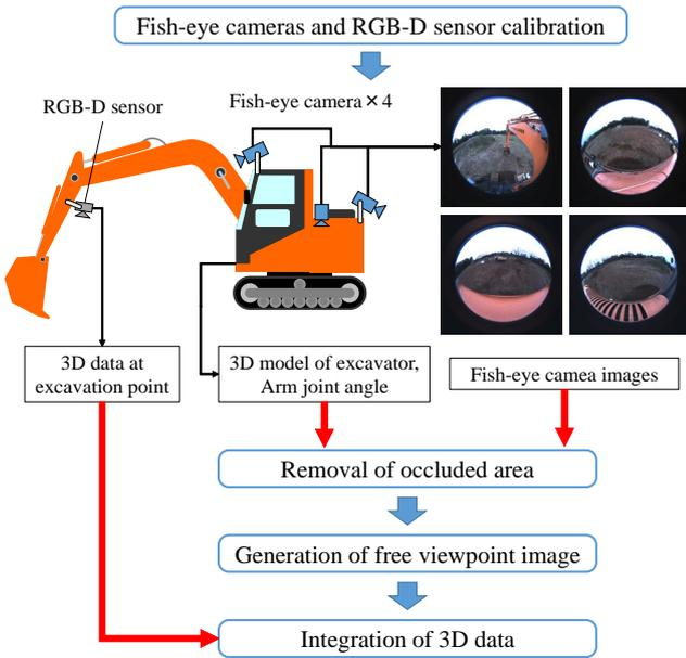
Fig. 4. Image generation process of proposed method.
