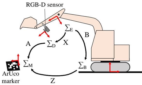
Fig. 10. Coordinate systems for RGB-D sensor calibration.
