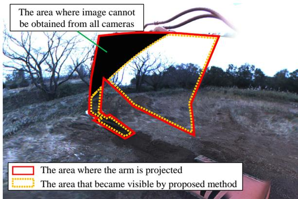
**Fig. 9.** Expanded region of field of view.
