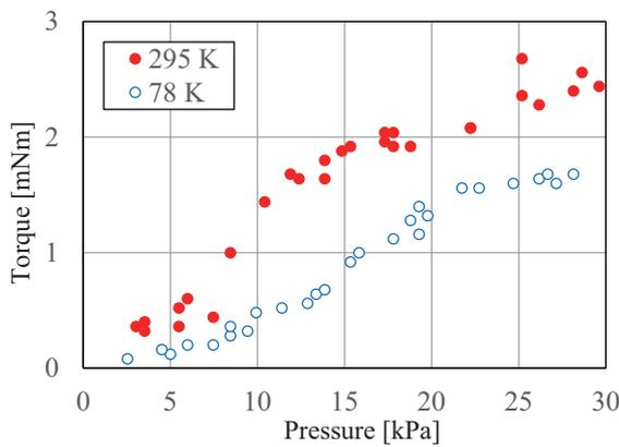
**Fig. 11.** Relationship between applied pressure and generated torque at different temperatures.
