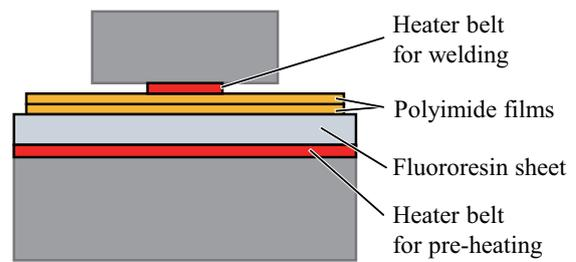
Fig. 1. Schematic view of PI welding machine.
