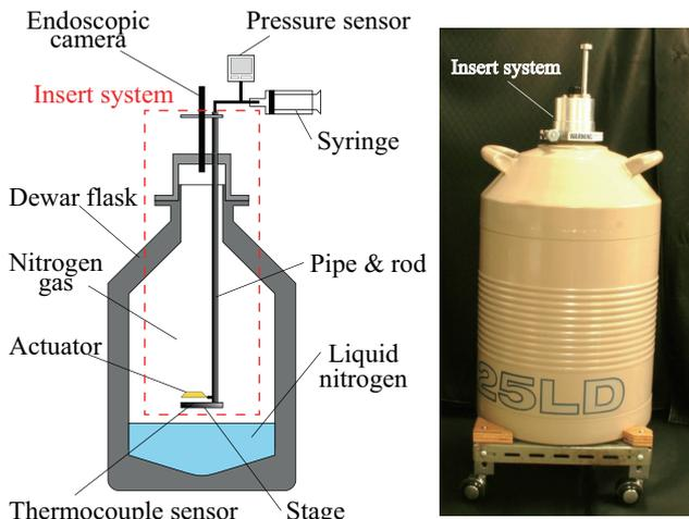
**Fig. 5.** Schematic view and photograph of evaluation system at liquid nitrogen temperature.
