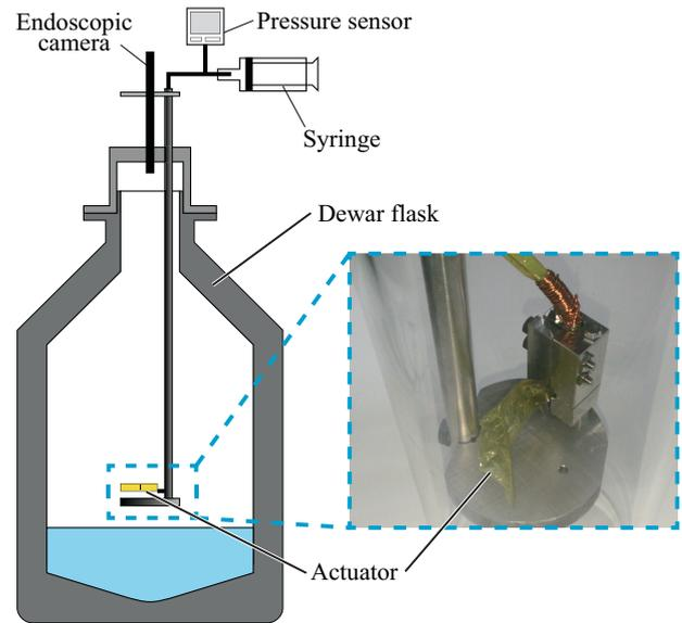
**Fig. 6.** Schematic view of setup for bending angle evaluation.
