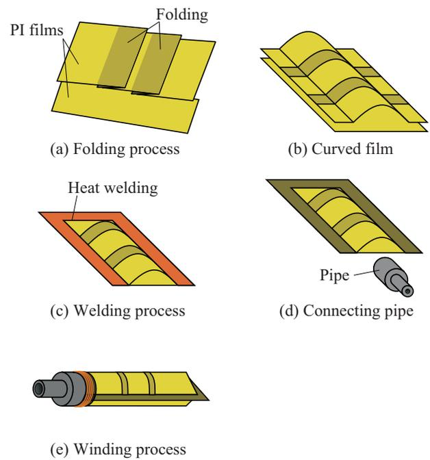
**Fig. 3.** Actuator fabrication procedure: (a) folding upper film, (b) curving pleated film, (c) welding three sides of two films, (d) connecting pipe to chamber, and (e) winding of chamber and pipe.
