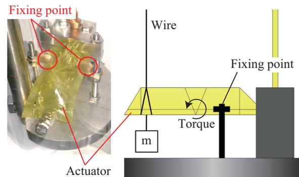
**Fig. 10.** Schematic view of around measuring point.
