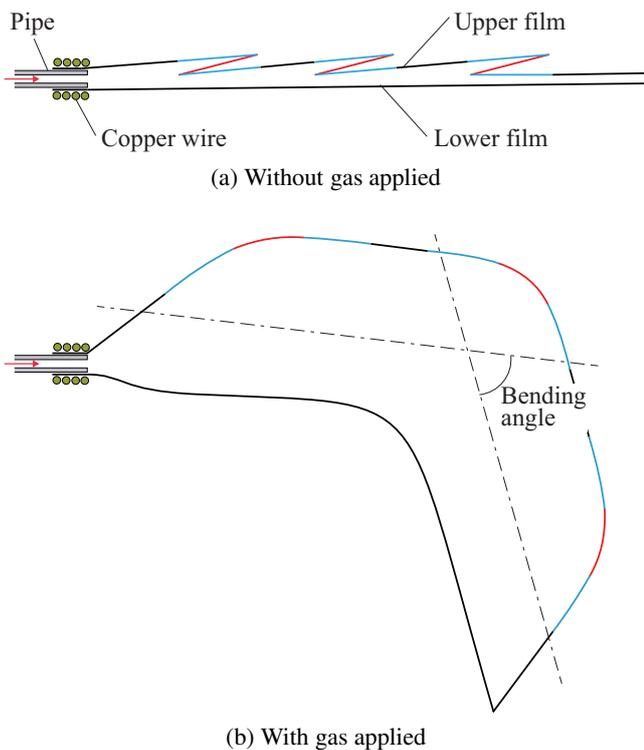
**Fig. 2.** Structure of soft actuator for use at liquid nitrogen temperatures.
