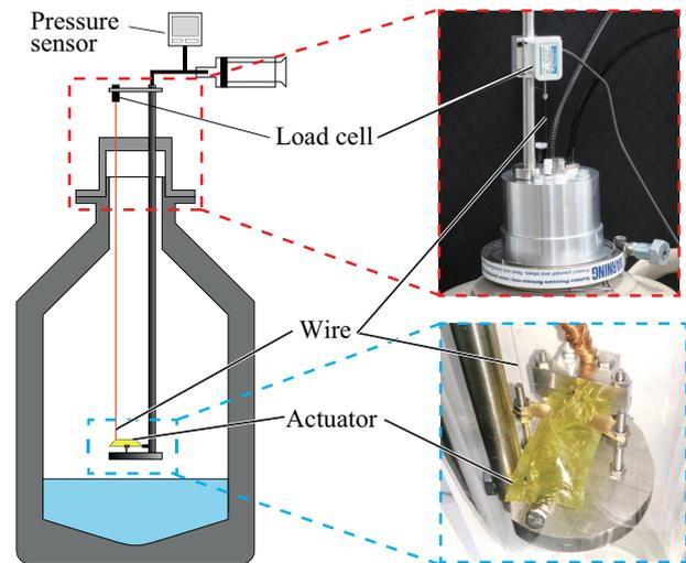
**Fig. 9.** Experimental setup for evaluation of generated torque.
