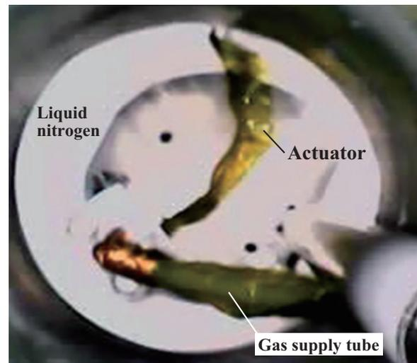
**Fig. 7.** Actuator bent inside Dewar flask (liquid nitrogen temperature environment).
