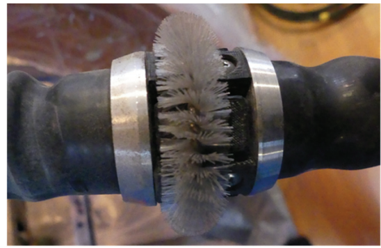
Fig. 45. Condition of the peristaltic duct cleaning robot after actual house cleaning.
