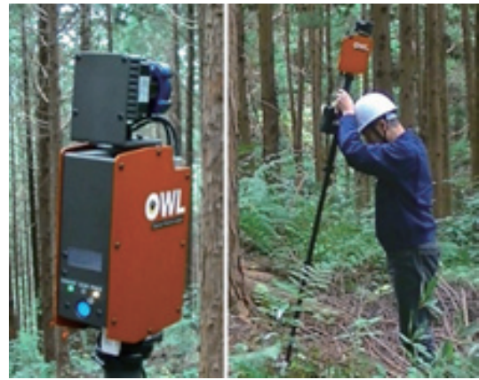
Fig. 1. A product of the scanner for forest measurements named OWL (Optical Woods Ledger) of AdIn Research, Inc. [27].
