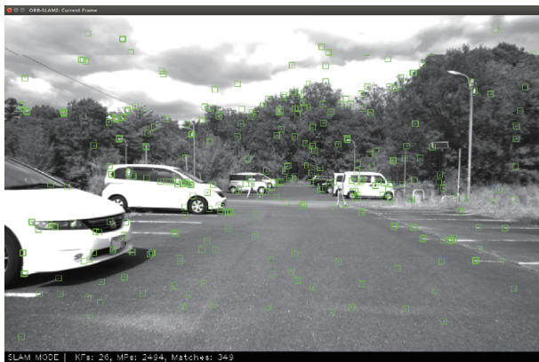
Fig. 8. An image example and ORB feature points (2).
