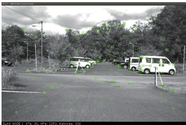
Fig. 9. An image example and ORB feature points (3).
