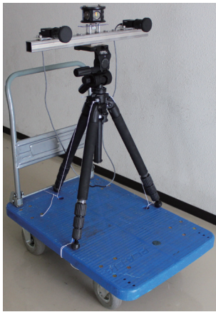
Fig. 3. A pair of the stereo camera and prism for tracking on a cart.
