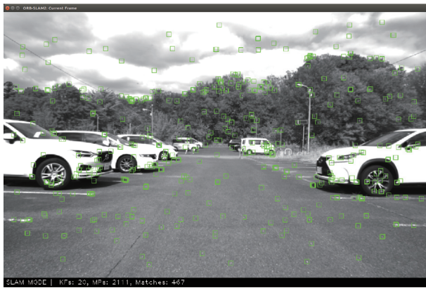
Fig. 7. An image example and ORB feature points (1).
