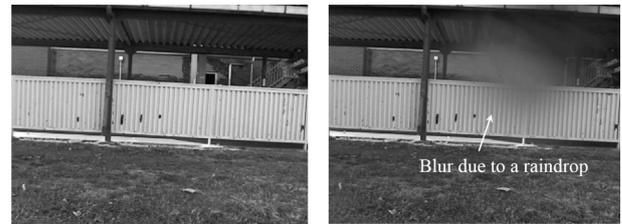
**Fig. 6.** Raindrop influence on a camera image. The image at left was obtained when waterproofing parts were used. Raindrops did not become attached to light receptors, so measurement is clear. In contrast, the unclear figure at right was obtained when waterproofing parts were not used.
