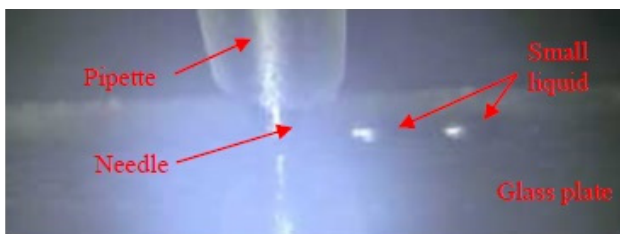
Fig. 17. Liquid at the tip of a needle is transferred.
