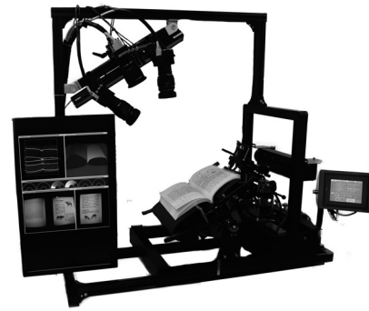
Fig. 17. BFS-Auto: high-speed high-resolution book digitization.
