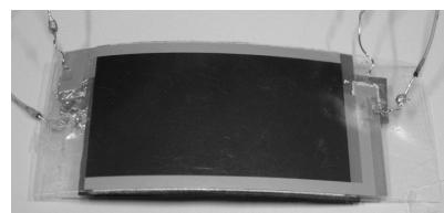
Fig. 9. High-speed tactile sensor.
