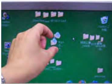
(a) Desktop manager operated based on user hand and finger movement.
