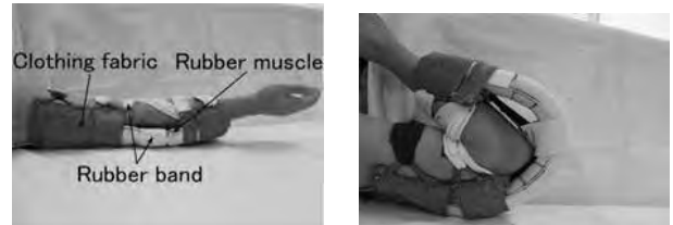
(a) Before pressurized (b) Pressurized to 250 kPa
