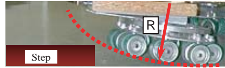
Fig. 10. Approximation of Omni-Disc as a large wheel.
