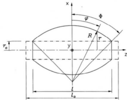
Fig. 8. Straight fibres muscle geometry
