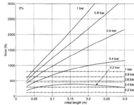
**Fig. 13.** Traction force of a straight fibres muscle (—) and a McKibben muscle (---) versus the initial length for different supply pressures (0% contraction ratio)
