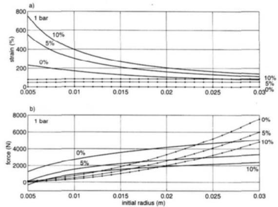
**Fig. 15.** Maximum chamber strain (a) and traction force (b) of a straight fibres muscle (—) and a McKibben muscle (↔) versus the initial radius, for different contraction ratios (1 bar supply pressure)
