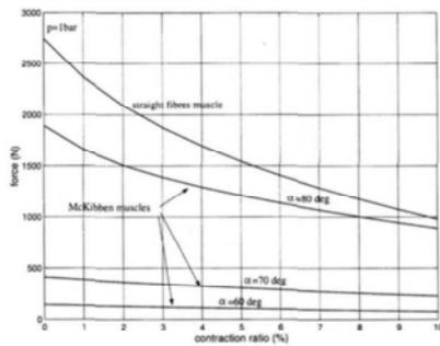
**Fig. 11.** Traction force of a McKibben muscle, for different winding angles, and of a straight fibres muscle versus the contraction ratio (1 bar supply pressure)
