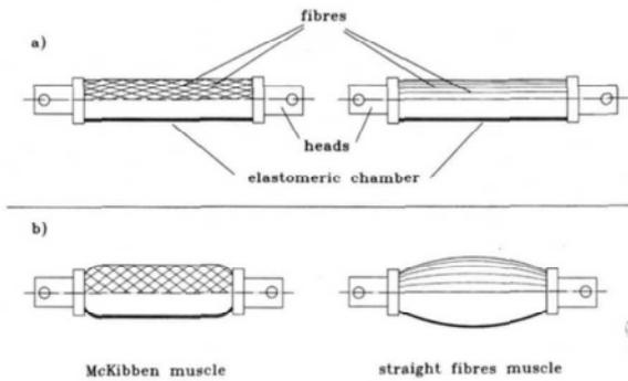
**Fig. 1.** Pneumatic muscle actuators. a) undeformed conditions. b) deformed conditions
