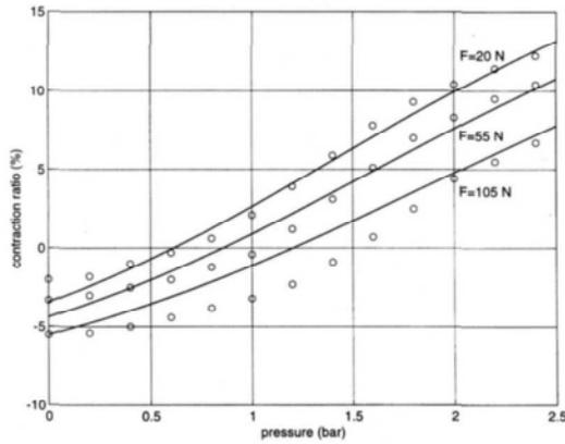
**Fig. 5.** Comparison between theoretical (continuous line) and experimental characteristic of McKibben muscle
