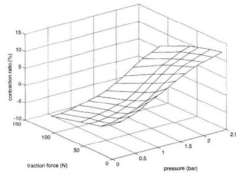
**Fig. 3.** Experimental contraction ratio of a McKibben muscle as a function of the traction force and the supply pressure.
