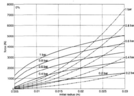
**Fig. 16.** Traction force of a straight fibres muscle (—) and a McKibben muscle (↔) versus the initial radius, for different supply pressures (0% contraction ratio).
