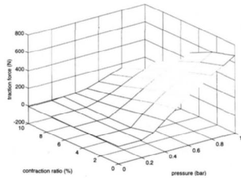
**Fig. 7.** Experimental traction force of a straight fibres muscle as a function of the contraction ratio and the supply pressure
