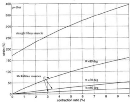
**Fig. 12.** Elastomeric chamber strain of a McKibben muscle, for different winding angles, and of a straight fibres muscle versus the contraction ratio (1 bar supply pressure)
