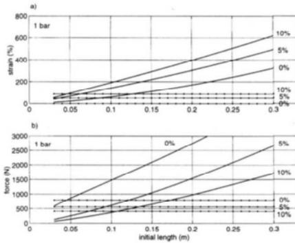
**Fig. 14.** Maximum chamber strain (a) and traction force (b) of a straight fibres muscle (—) and a McKibben muscle (↔) versus the initial length, for different contraction ratios (1 bar supply pressure)
