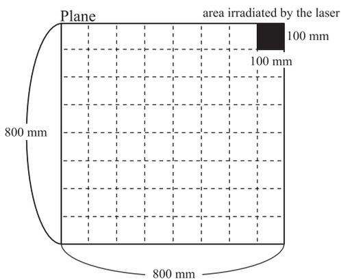
**Fig. 3.** Areas irradiated by the laser in a target plane. The filled area shows the area that the laser can irradiate at one time.
