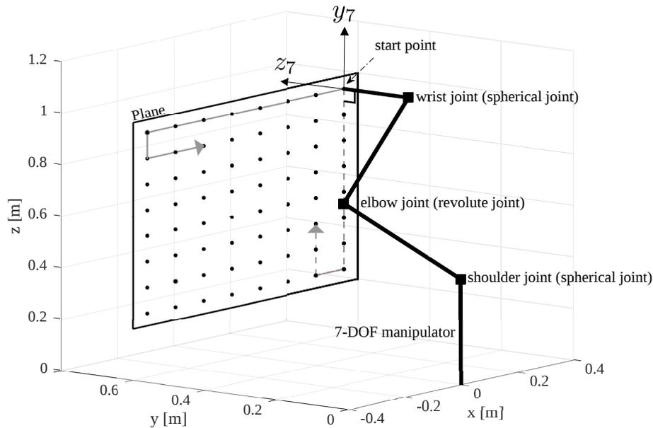
**Fig. 2.** Sequential reaching task on a plane. The circle points show the target points. The gray solid and dashed lines show routes based on the horizontal direction and the vertical direction, respectively. The squares show the Spherical-Revolute-Spherical joints of the 7-DOF serial link manipulator.
