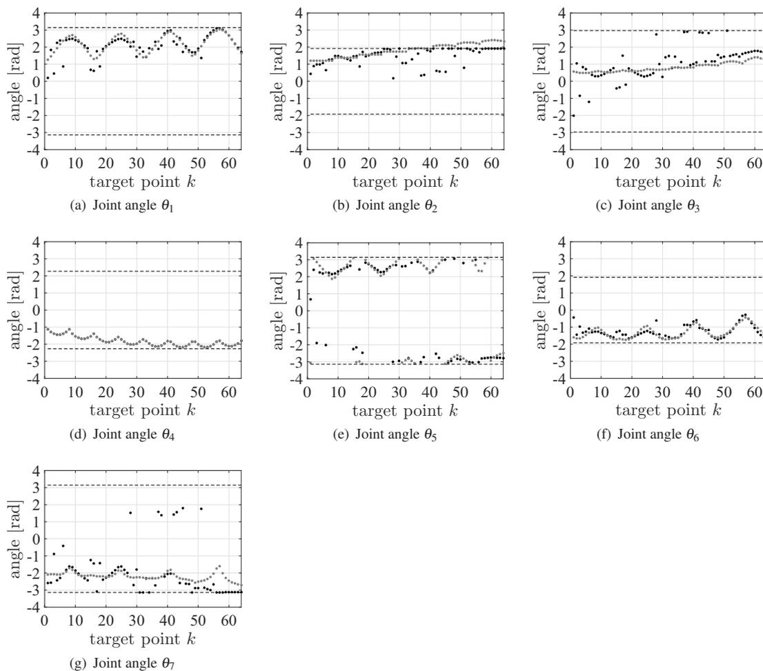
**Fig. 5.** Trajectories of joint angles of solution No.7 along the horizontal route. The black and gray dotted lines show the optimal solution based on the minimum Euclidean distance and the inverse kinematic solution, respectively. The dashed lines show the lower bounds and the upper bounds of the joint angles. Note that the fourth joint angle is the same in the inverse kinematic solution and the optimal solution because the joint angle is independent of the arm angle.
