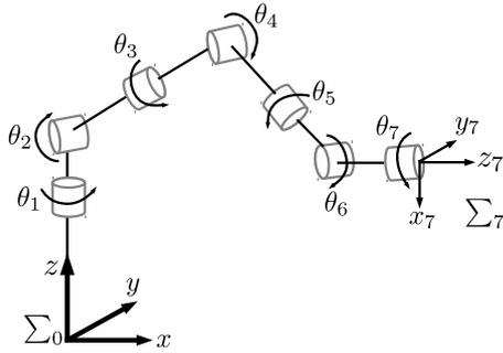
Fig. 1. 7-DOF serial link manipulator.
