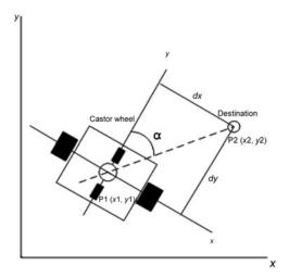
Fig. 2. Model of the OmniBot.
