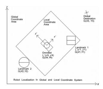
Fig. 9. Localization of the OmniBot by using landmarks.
