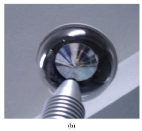
**Fig. 4.** (a) Side view of the camera-mirror system and (b) the mirror on the omni-directional camera.
