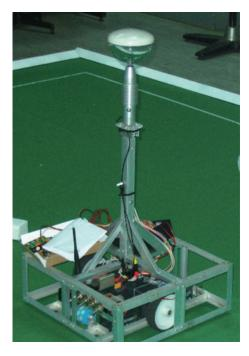
Fig. 1. The OmniBot using differentially driven wheels.
