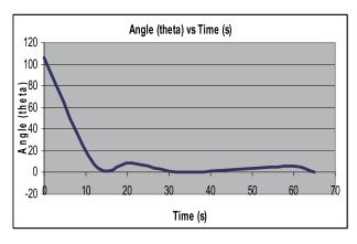
Fig. 12. Graph of heading angle against time.
