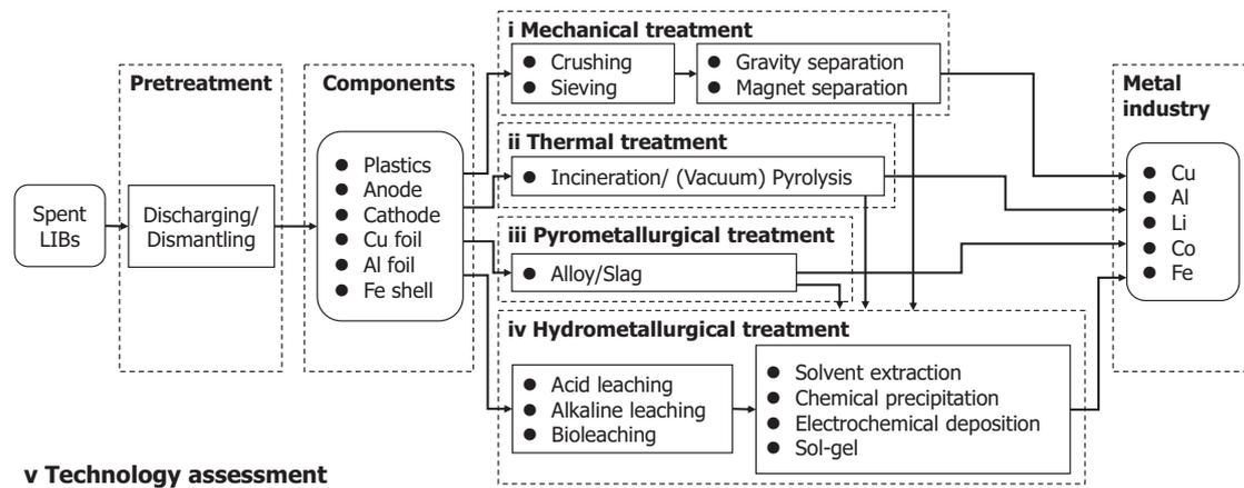
Fig. 3. Possible technology combinations for recycling spent LiBs with the contents of Subsection 3.2.2.
