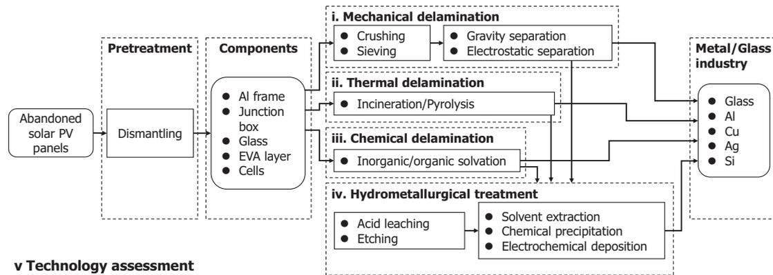
**Fig. 2.** Possible technology combinations for recycling abandoned solar PV panels with the contents of Subsection 3.2.1.
