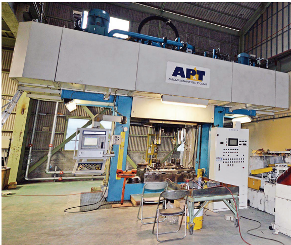
Fig. 3. Appearance of hydraulic press with six cylinders.
