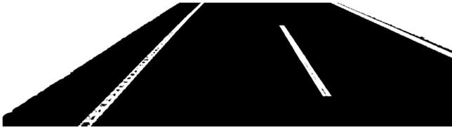
(a) The result of lane mark detection with precise road surface region.
