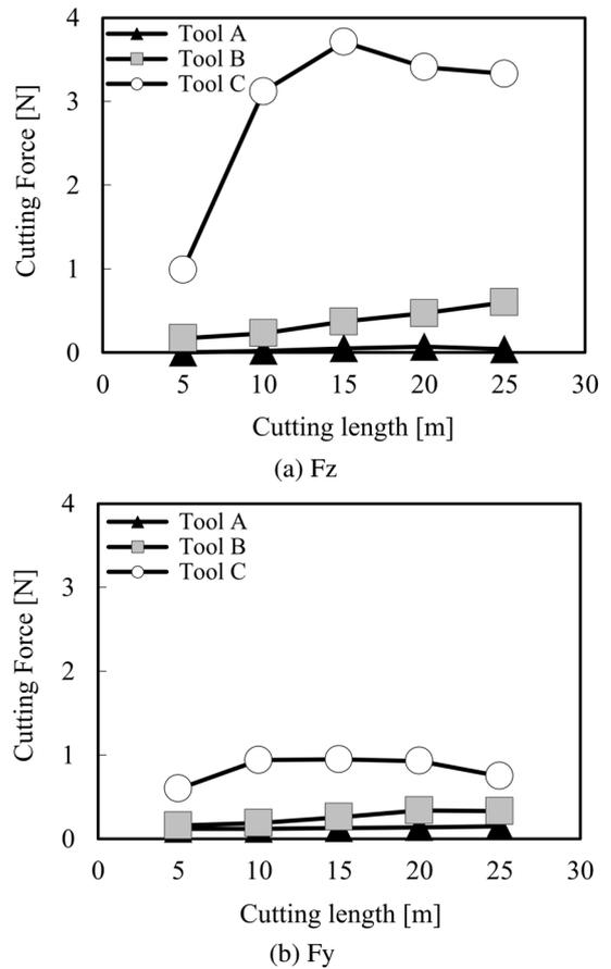
Fig. 8. Relationship between cutting force and cutting length.
