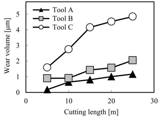
Fig. 6. Relationship between wear volume and cutting length.
