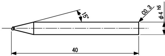
Fig. 1. Binderless CBN end mill.
