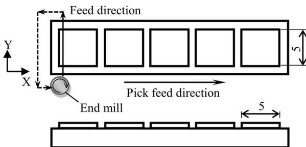
Fig. 3. Definition of tool path.
