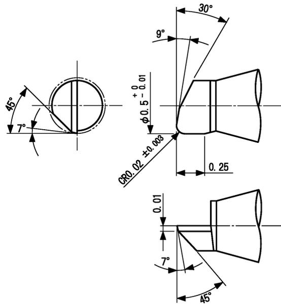
Fig. 2. Cutting edge shape of the end mill.
