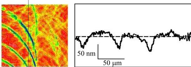
Fig. 11. Cutting surface on heat-treated steel.
