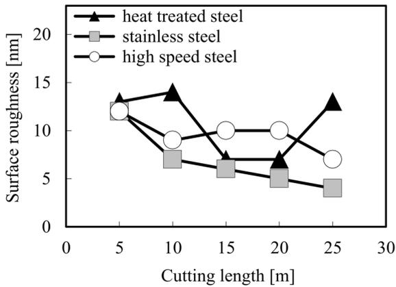
Fig. 10. Relationship between surface roughness and cutting length.
