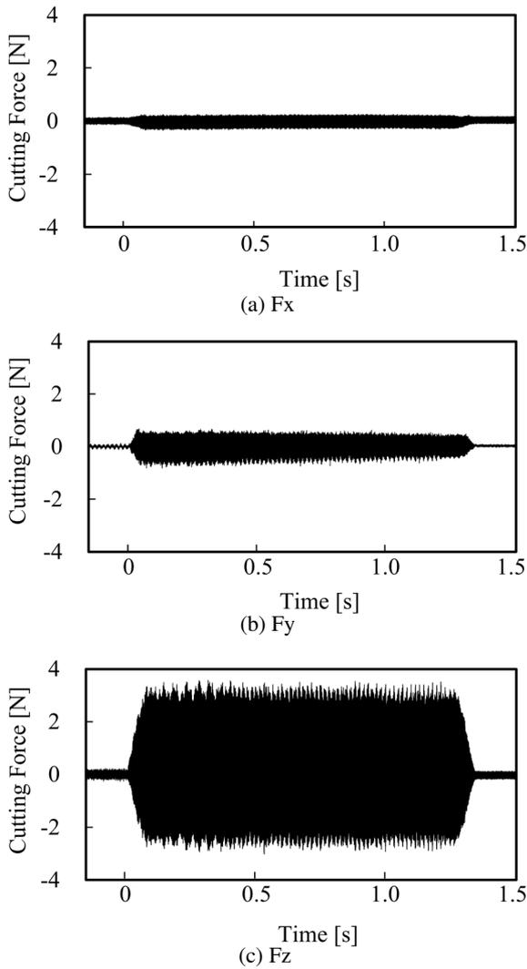
Fig. 7. Cutting force in end milling of the high-speed tool steel.
