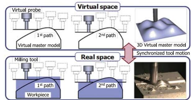
**Fig. 2.** Real-time tool path generation in Digital Copy Milling (DCM).
