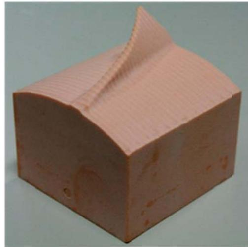
**Fig. 14.** Product shape finished under tool posture control.
