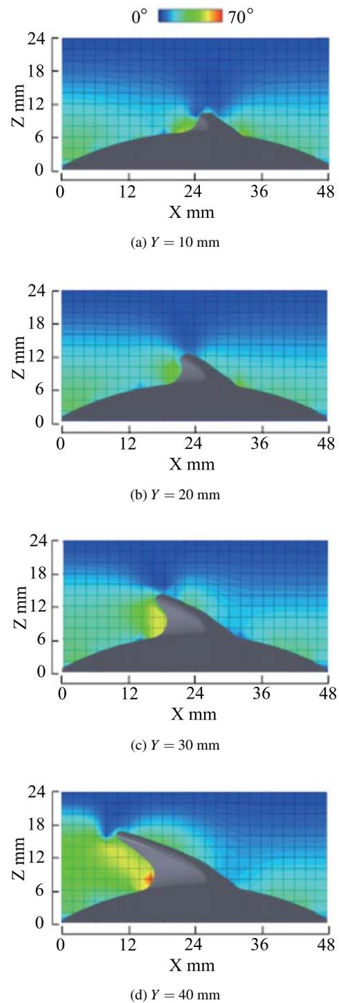
Fig. 12. Tool posture distribution for tool posture control.
