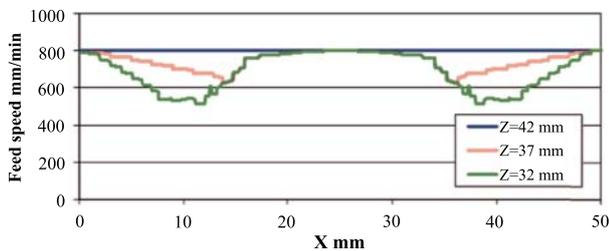
**Fig. 9.** Feed speed transition during milling operation (scanning-line mode along the  $X$  axis at  $Y = 24$  mm).
