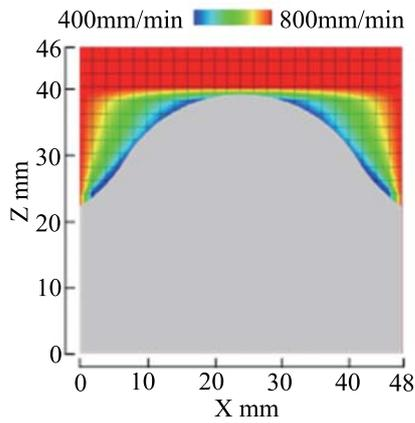
**Fig. 8.** Feed speed distribution for feed speed control ( $x-z$  plane at  $Y = 24$  mm).
