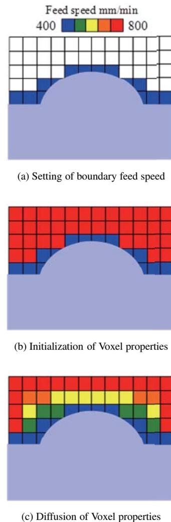
Fig. 4. Setting the voxel properties for feed speed control.
