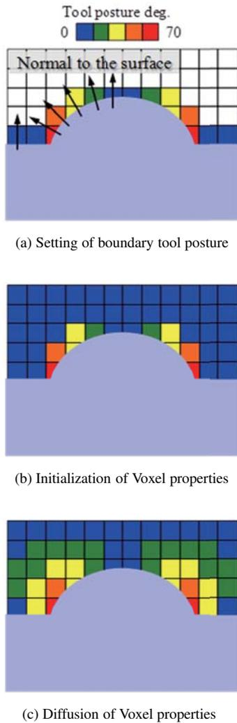
Fig. 6. Setting the voxel properties for tool posture control.
