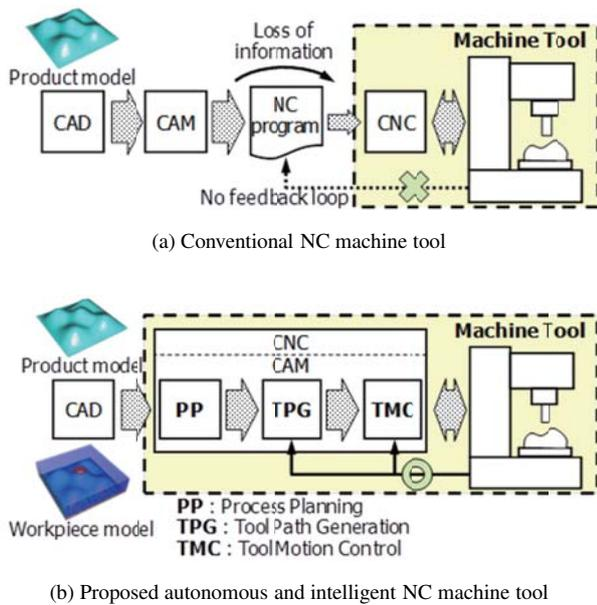
**Fig. 1.** New concept to realize an autonomous and intelligent NC machine tool.
