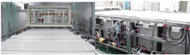
Fig. 3. Electroless nickel plating equipment.
