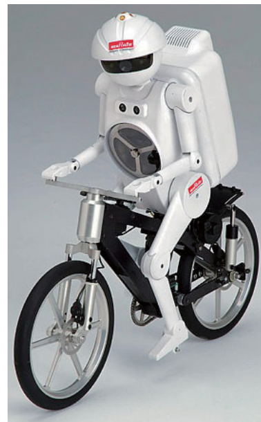
Fig. 1. Murata Boy [5], self-balancing bicycle riding robot.
