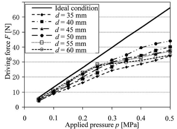
Fig. 12. Experimental results of driving force.
