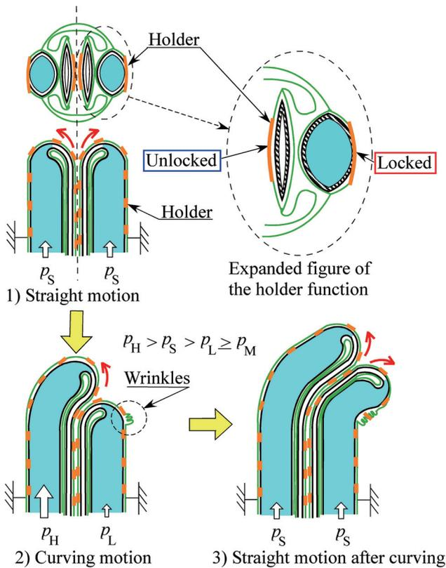
Fig. 8. Steering the direction of tip.
