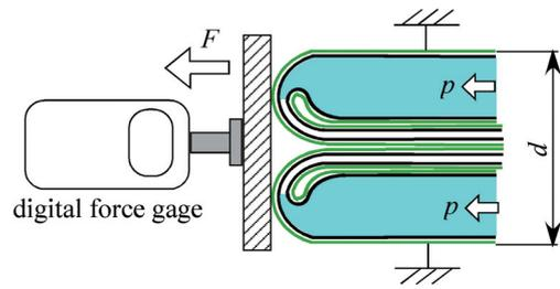
Fig. 11. Experimental setup to measure the driving force.
