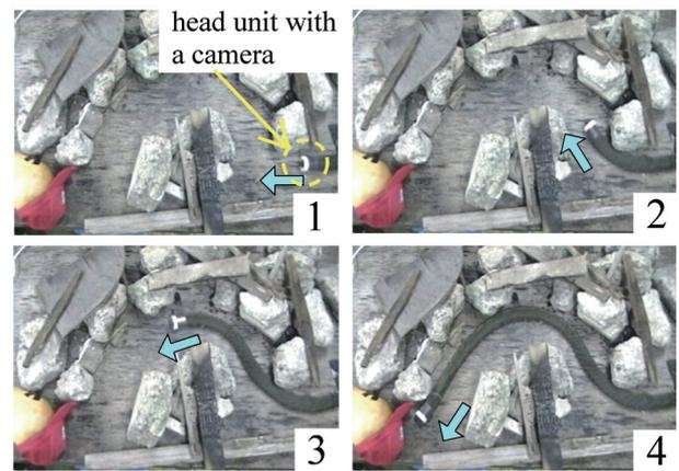
**Fig. 14.** Experimental results of Grow-hose-I steering in the narrow path.
