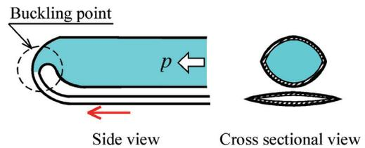
**Fig. 4.** Driving principle using the buckling phenomenon on a flat tube.
