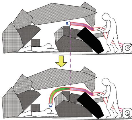
**Fig. 3.** Search using actuator extension with a camera at a disaster site.
