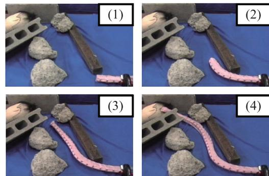
Fig. 2. Tip growth in the initial prototype steering along a curved path.
