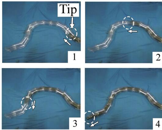
**Fig. 13.** Experimental Grow-hose-I results in a pipe with an inner diameter of 70 mm.
