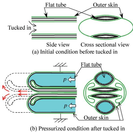
Fig. 6. Tip growth with two flat tubes facing.
