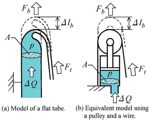
Fig. 7. Tube model (left) and its equivalent (right).
