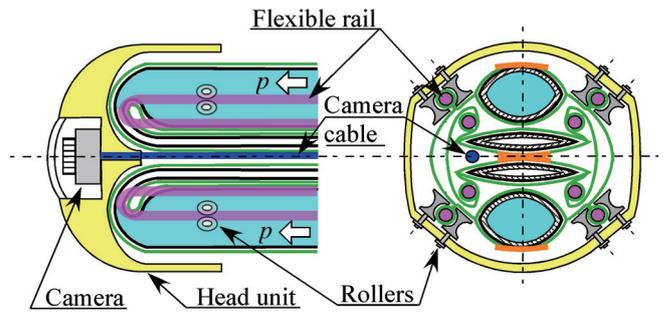
Fig. 9. Head unit with a camera.
