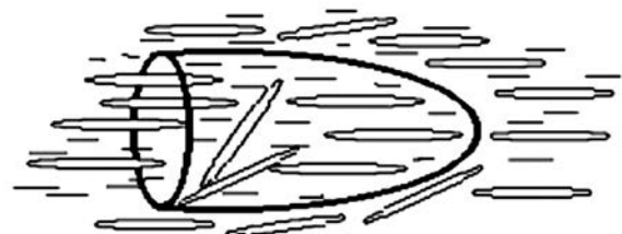
Magnetic pin media rotate and enter into contacts with the works
