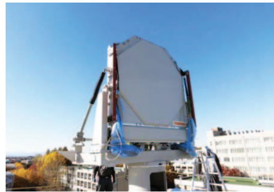
Fig. 5. A Multi-Parameter Phased Array Weather Radar (MP-PAWR) by TOSHIBA (see [13]).
