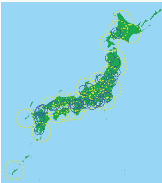
Fig. 3. Location of radar observation by MLIT. Dashed and solid circles indicate C-band and X-band radars, respectively.
