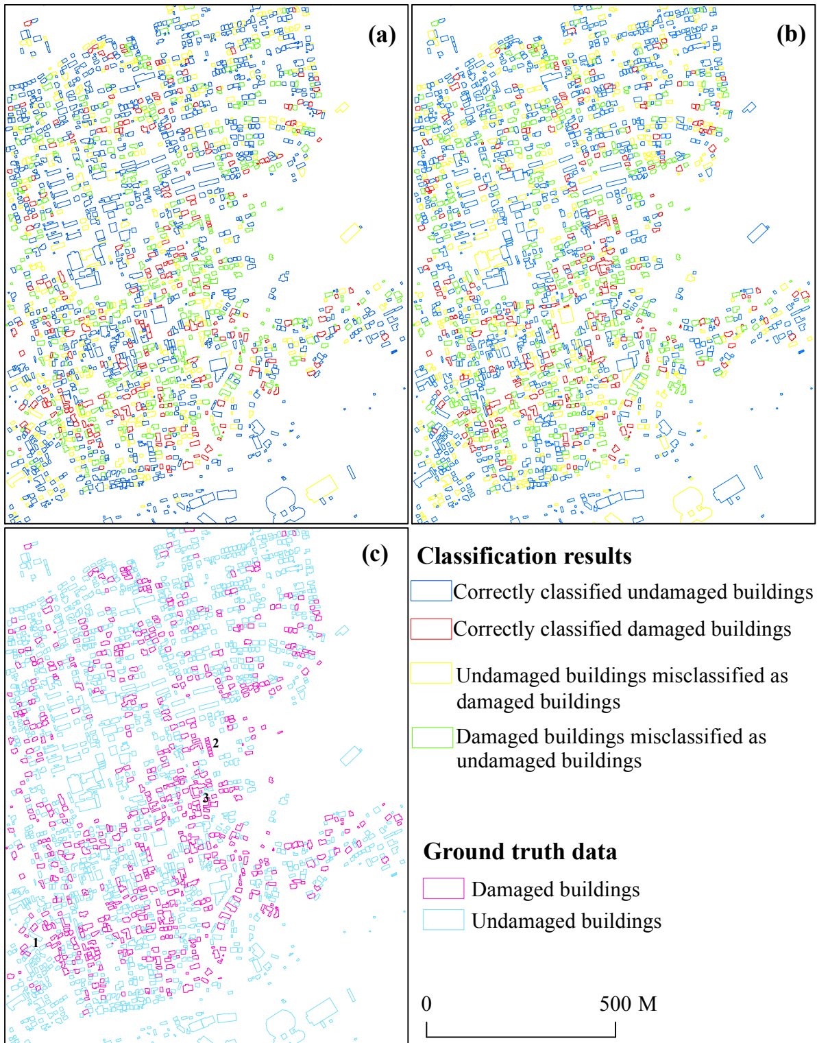
Fig. 5. Results of building damage classification using the K-Nearest Neighbors classifier: (a) damage mapping result using only the post-event SAR image; (b) damage mapping result using multi-temporal SAR images; (c) ground truth data in our study area. Note: numbers 1, 2 and 3 in Figs. 5(c) represent the positions of buildings in Figs. 6(a) , 6(b) and 6(c) , respectively.
