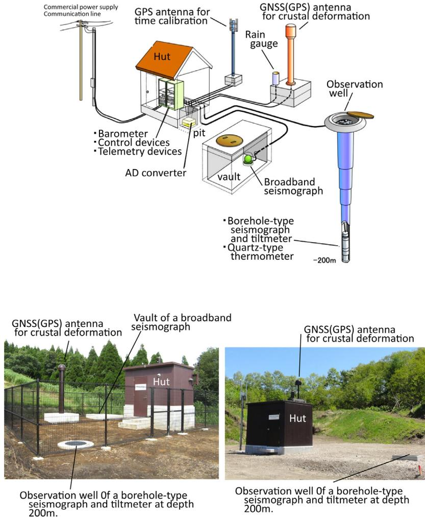
**Fig. 2.** Conceptual diagram and photograph of V-net station. The left photograph shows the Asosan V-net station in the Kyushu area. The right photograph is the Hokkaido-Komagatake V-net station in the Hokkaido area.
