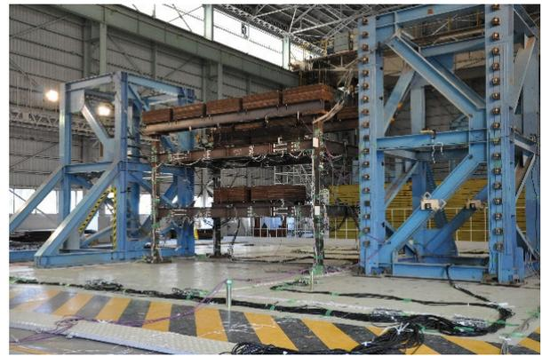
**Fig. 1.** Small-scaled steel frame specimen.
