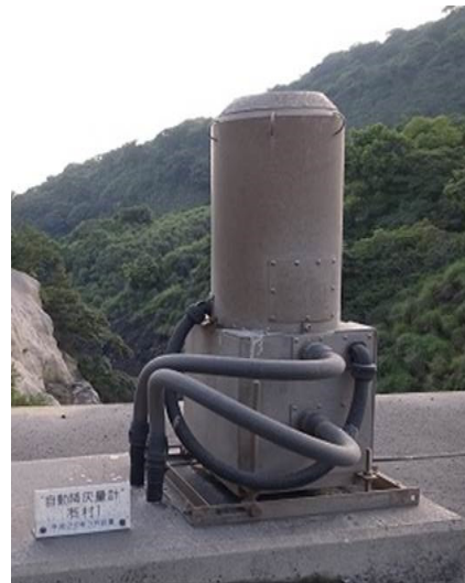
Fig. 11. Automatic weight measurement system for volcanic ash.
