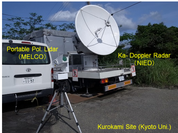
Fig. 2. NIED Ka-band Doppler radar and portable polarization Doppler lidar at Kurokami observation station (L2 in Fig. 7) of Kyoto University in Sakurajima.
