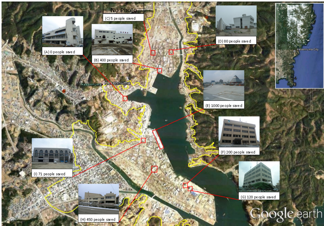
Fig. 2. Map and images of nine vertical evacuation buildings in Kesennuma City, including numbers of people saved and tsunami inundation marked in yellow [29]. These comprise office buildings (A, F, G, I); a cannery (B), a retail building (C), welfare centre (D), a car parking deck (E) and a community centre (H).
