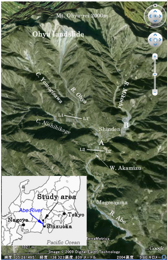
Fig. 1. Showing the around terrain of study area (using Google Earth) 'A' is the river junction of Ohya River and Mikochi River where the landslide dam was formed. 'B' shows that the pond was here in the past.
