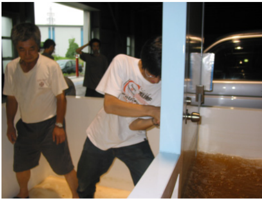
Fig. 23. Evacuation experiment by use of door model.
