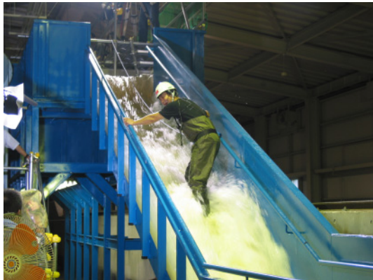
Fig. 19. Evacuation experiment by use of staircase model.
