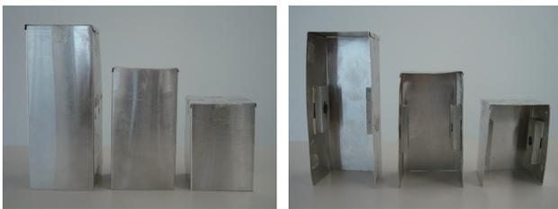
**Fig. 2.** Above from left to right at left, are the fronts of the large, medium, and small PAOs and, from left to right at right, their backs. Two rectangular metal pieces with holes in the center are attached to the inside of the left and right sides of each box. Holes help tie the box to the force sensor.
